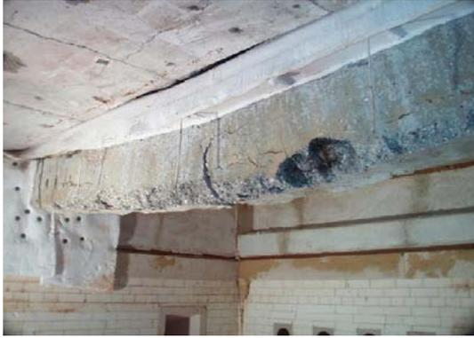
**Fig 8** Rupture at the mid centre of the concrete in beam 1 after fire test
