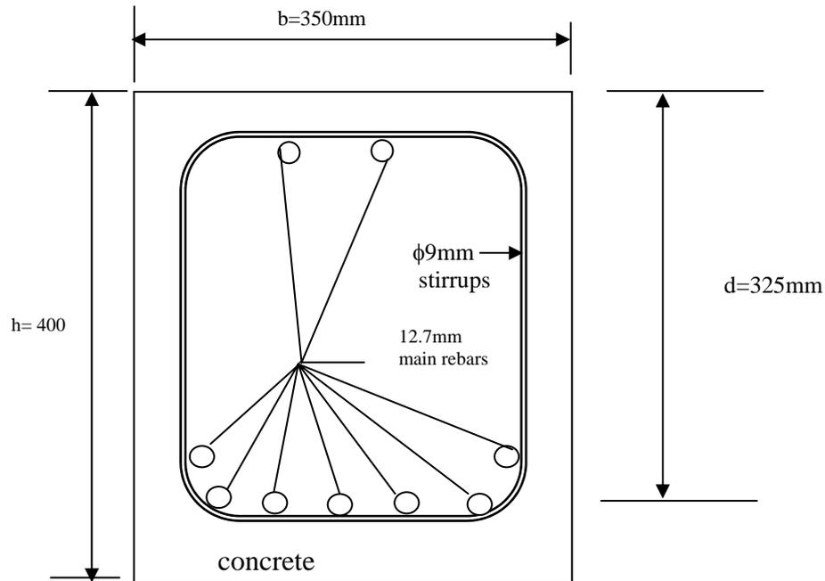
**Fig 1b** Beam cross section with reinforcement arrangement
