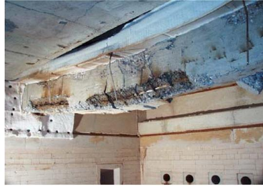
**Fig 9** Failure of beam 2 after fire test inside the furnace shows some flexural cracks and rupture in the main reinforcement
