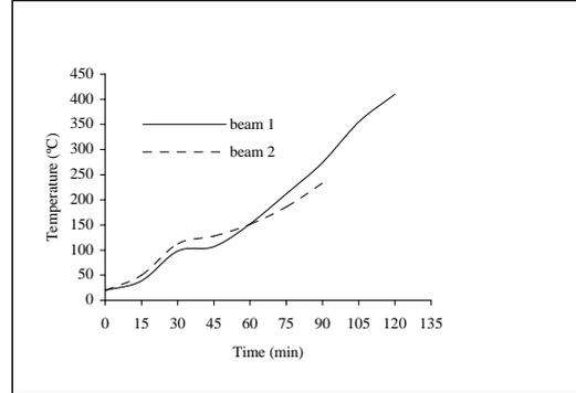
**Fig 12** Average stirrups temperature in beam 1 and beam 2
