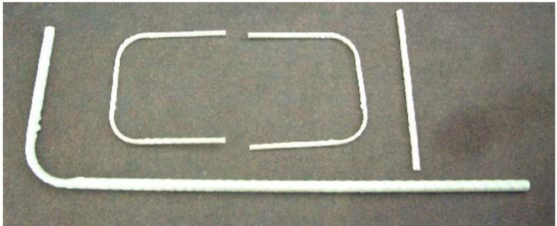
**Fig 1a** GFRP rebar shapes used as reinforcement for control beam and beam 1
