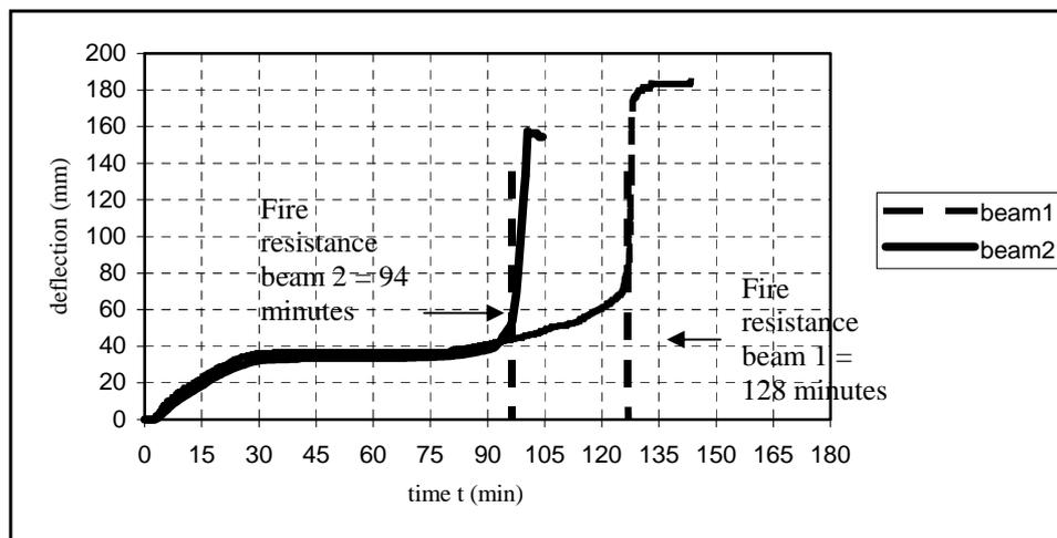
**Fig 7** Heating time-deflection curves for beam 1 and beam 2
