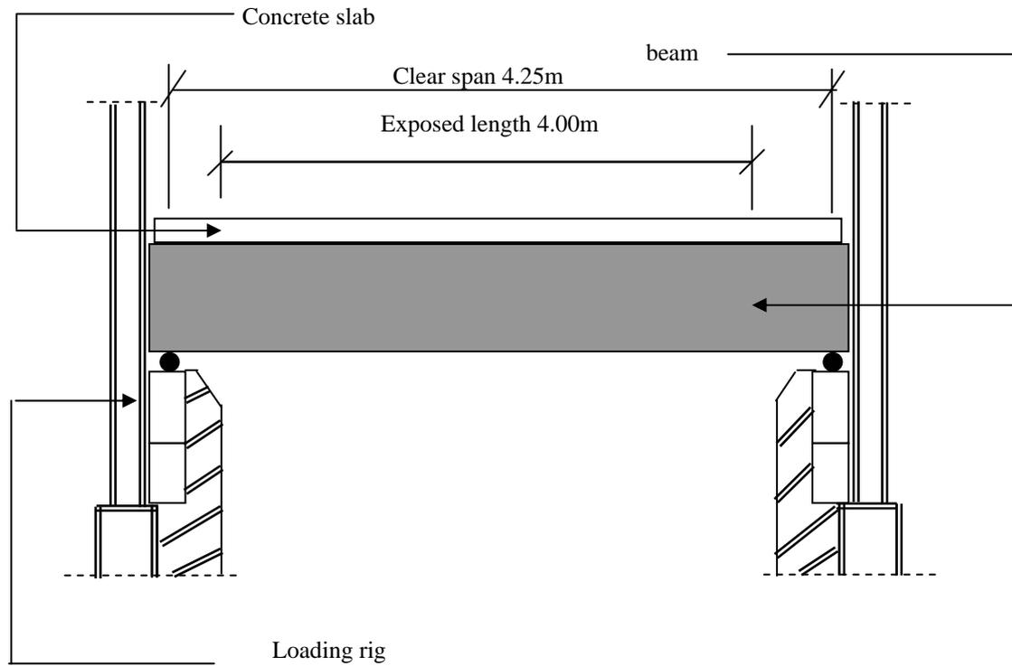
**Fig 6** Fire test set up
