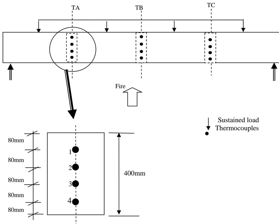
**Fig 4** Thermocouples embedded in concrete. Group of thermocouples at A, B and C in concrete Nos. 1-4 at centre line 80mm c/c ( $3 \times 4 = 12$ ).
