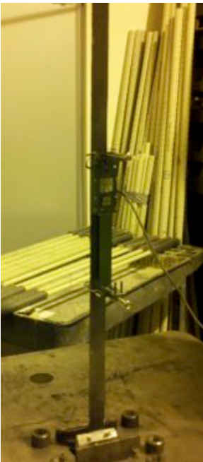
Aslan 400 Laminates with extensometer and after valid tensile test
