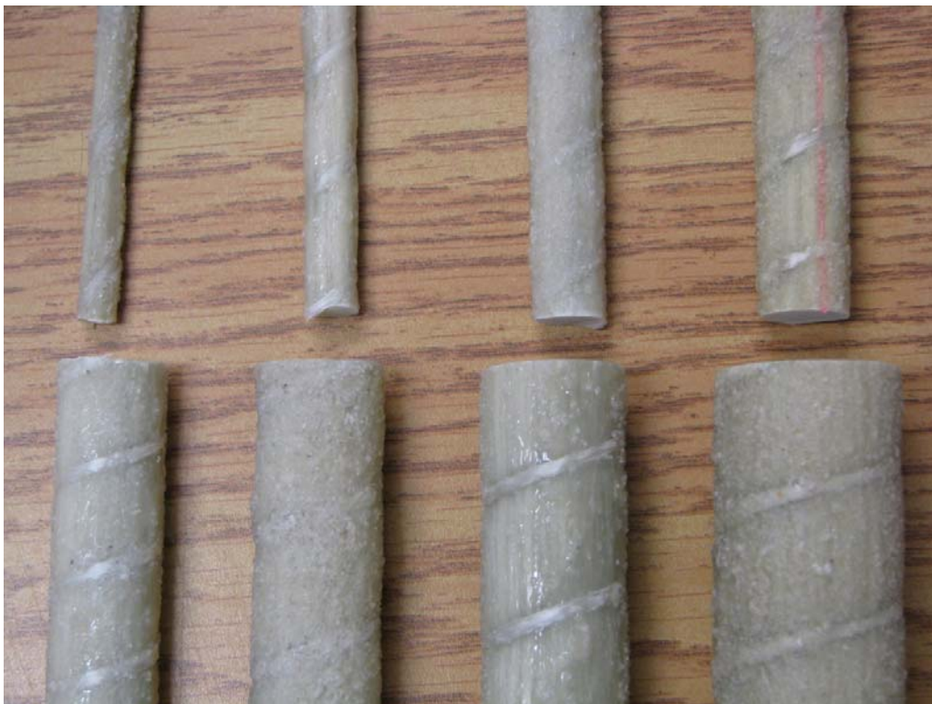
Figure 1: Tested Aslan GFRP bars No. 2, No. 3, No. 4, No. 5, No. 6, No. 7, No. 8, and No. 10
